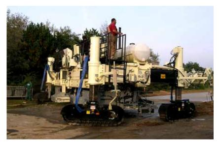
The S850 is equipped with counter-rotation capability where the operator can quickly re-orientate the S850 crawlers into the counter-rotate position and rotate the machine 360 degrees within the machine's overall width. Counter-Rotation is just one of the pre-programmed steering modes available with the S850 controls, along with crab and coordinated steer, front and rear only steer.
