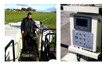
visibility of the paver's concrete spreading operation. The control desk includes a lock out / power switch located inside the control desk, an aluminum cover for weather and vandal protection and an emergency stop.
