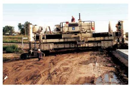
Optional 90 Degree Steering allows the four crawler tracks to be turned perpendicular to the paving direction with a flip of a switch. There is a limited steering range in this mode. 90 Degree Steering reduces the size of hand pours, dramatically increasing on site paver maneuverability and helps speed width change and self-loading for transport.
