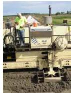
The S850 features superb operator visibility. The operator can easily see all around the machine including under foot into the concrete liquification hopper. The Operator Control Desk is centrally located on the tractor center module to optimize visibility as well. The S850 is provided with emergency stops on all four corners of the machine with magnetic holders to allow them to be relocated.
