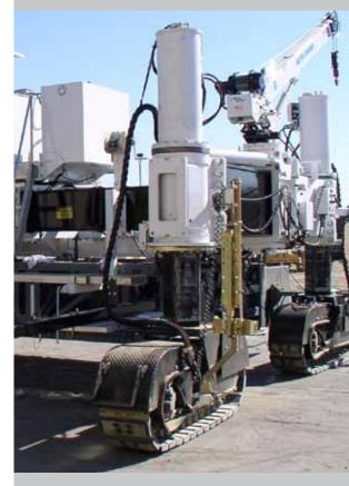
G&Z's precision built, square-to-round style jacking column design with builtin replaceable bronze wearing parts that prevent sticking allow for the most positive steering control in the industry. This design also offers years of precise, maintenance free use.
