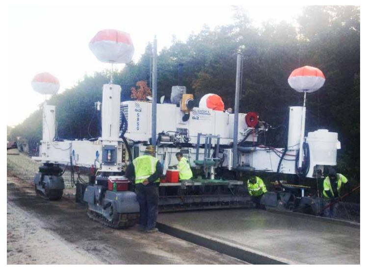
The G&Z **S850SL** (Swing Leg): Concrete Slipform Paver is the newest addition to G&Z's line of concrete paving products. With the success of the S600 paver and its productivity features, the popular and patented **AccuSteer** and **SmartLeg** are now available options on G&Z's reliable and time tested S850 Paver in lieu of the QUADRA Bolster system.
