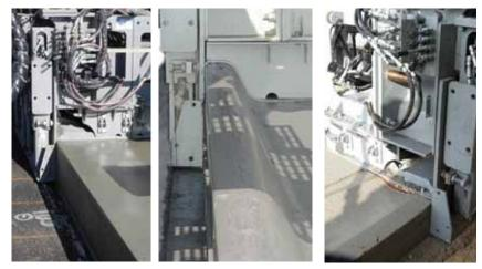
The terminal pan sections on the Paving Kit are provided with edge overbuild adjustment to help compensate for edge slump. The terminal pans can be substituted with other optional integral curb and gutter mold cross sections.
