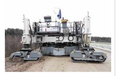
AccuSteer greatly enhances job site maneuverability in the tightest of confines and minimizes the size of hand pours with its 90 degree steering capability.
