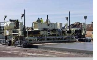
Deep section, fabricated, tube type construction of the double telescopic tractor frame design allows paving widths from 12 ft. (3.66 m) to 26 ft. (7.92 m). The machine telescopes 7 ft. (2.13 m) on either side of the 12 ft. (3.65 m) center module for a total telescopic ability of 14 ft. (4.27 m) With the addition of optional bolt-in frame sections, the total possible paving width is 42.5 ft. (13 m).
