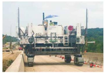
SmartLeg dramatically reduces the time needed to cross narrow bridges by using the hydraulic cylinders to swing the legs inboard positioning the crawler track inside the edge of concrete.
