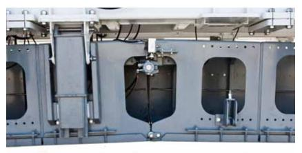
The optional Paving Kit Crowning Section is provided with a hydraulic motor driven, dual screw jack system that holds the crown position without drift. A digital readout of the crown angle is provided at the operator console. Computerized Crown / Transition Control system is also available as an option.
