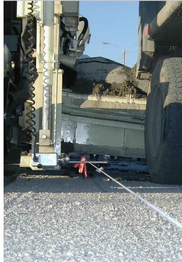
Electronic, no contact type, moisture proof, and proportional Sauer Danfoss (SD) steering and elevation sensors, as well as G&Z's own proprietary software provides precise steering and elevation accuracy and self-diagnostic capability.
