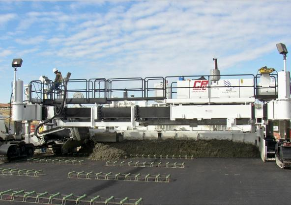
The PS1200's heavy duty tractor frame with 7'-0" (2.13 m) telescopic ability capable of 18'-0" to 25'-0" (5.50 m to 7.60 m) spreading widths. With extensions, spreading widths of up to 41'-0" (12.5 m) are possible. Its narrow profile design requires only 25" (635 mm) of trackline. A telescopic hose/cable tray is provided for paving widths from 18'-0" to 29'-0" (5.50 m to 8.80 m). Extensions are available for narrower working widths.
