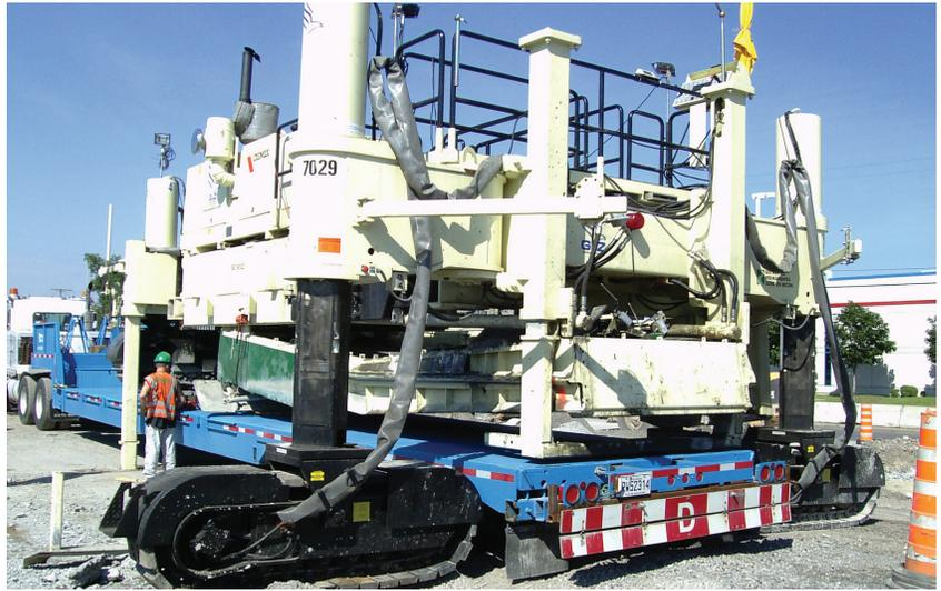
The PS1200 is designed to be transported in a single load. The PS1200 can self-load by walking over the top of the deck of a special trailer or self-load by straddling a trailer. With optional rotary actuator steering, the four track PS1200 can walk and steer on a trailer with a removable gooseneck. To reduce weight for interstate transport, the Strike-off / Spreader Plow module as well as the conveyor can be removed.
