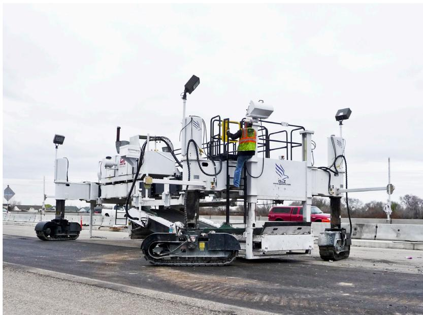
The standard PS1200 can be manually or automatically steered by varying the speed of the tracks on one side of the machine in relationship to the other. One side of the machine may be operated independently from the other allowing the placer operator tremendous flexibility for maneuvering in tight confines including counter rotation capability.
