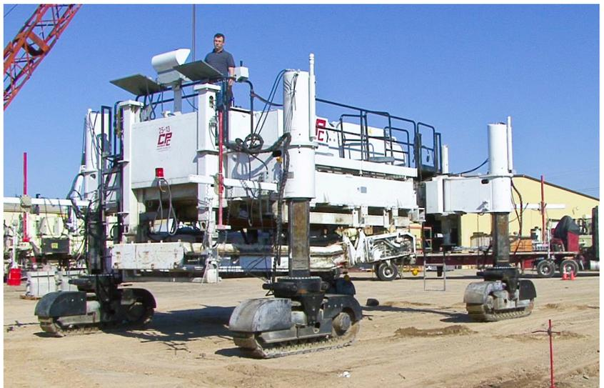
Optional 90 Degree Steering allows the four crawler tracks to be turned perpendicular to the paving direction with a flip of a switch. There is a limited steering range in this mode. 90 Degree Steering reduces the size of hand pours, dramatically increasing on site placer maneuverability and helps speed width change and self-loading for transport.
