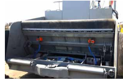
Hinge Up Flop Gate with Shuttle Plate (patent pending)
