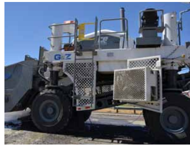
Swing Open Side Panels for Cleaning Access
