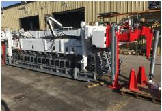
G&Z's DBI accurately inserts dowels in concrete behind the slipform confining pan. The unique combination of the DBI confining pan, trailing sideforms and vibrating forks ensure good consolidation and homogeneous concrete around the inserted dowel bars even with low airport slump concrete. This is accomplished while minimising the disturbance to the surrounding concrete surface during insertion.
