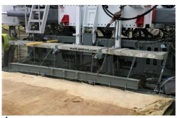
For extra smoothness, the S600 can be fitted with G&Z's Trailing Finishing Pan (TFP). The 48" (1.2m) wide TFP with fixed edger pans provides a proven method of finishing the pavement surface with fine adjustment ensuring sharp edges. It also accommodates a wide range of side bar inserters.
