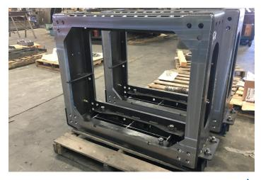
The Paving Kit's precision machined, box frame sections are rigid enough to achieve excellent smoothness results on projects with strict smoothness requirements. It can be provided with one or more crown sections. Thick flanges allow fewer bolts per section which speed width changes. The Paving Kit can be mounted in multiple locations under the S600 tractor and can be quickly and easily mounted or unmounted from the tractor.
