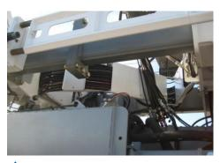
The patented VariWidth, double telescopic tractor frame, with single stage telescoping per side, allows 14ft (4.27m) of telescopic ability, the widest range in the industry. This is made possible by G&Z's patented tunnels through the bolsters. The heavy duty construction along with adjustable cam rollers and optional hydraulic clamping pucks ensures the tractor frame is rigid and without deflection.
