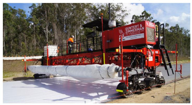
Polyethylene Paper Dispenser (Poly-Roll) can be supplied to protect the slab from rain. The support arms off main frame are equipped with adjustable turnbuckle to adjust height. The arms hinge up for transport. The spool with polypaper is hydraulic motor powered for fast lay down and pick up of the polyurethane paper. The TC1500 can hold up to 500 ft. (152 m) of polypaper on the spool depending on the width of the slab.
