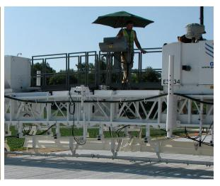
Electronic, no contact type, moisture proof, and proportional steering and elevation sensors, as well as G&Z's own proprietary software ensures steering and elevation accuracy. Sensor support arms are provided which hinge out to reach the grade wire location and hinge in for transport. Two steering sensors are provided, one located at the front and rear of the machine for forward and reverse steering, and are mounted on the same adjustable sensor support columns as the four elevation sensors.
