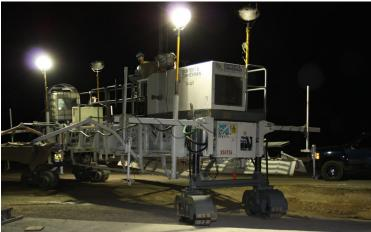
The TC1500 is available as an option with four tracks which offers the best possible weight distribution and lowest ground pressure, even in soft trackline conditions. The four track configuration also gives you a "flip of the switch"  $90^{\circ}$  steering feature which is a huge productivity booster. It speeds maneuvering / steering around the job site, self-loading / steering on and off a trailer, crossing bridges, and reduces hand pour sizes.
