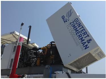
The Power Unit houses the diesel engine while providing The Power Unit's hinge up fiberglass enclosure provides excellent access to the pumps and filters for ease of monitoring, outstanding protection against the elements. Double vibrating service, and troubleshooting. The diesel fuel tank and hydraulic isolation on the engine / pump group and the insulated enclosure
