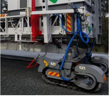
Optional telescopic support stands clamp anywhere along the main frame for ease of width change and transport. To change width, the support stands are telescoped to the ground on top of a skid plate and crawler tracks are turned 90° to walk the machine frame, together or apart, to allow a main frame section to be quickly added or removed. A pin is provided between the crawler tracks and jacking column yokes to prevent the track from rotating when relocating end tracks or changing width.
