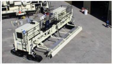
The TC1500 has counter-rotation capability like all G&Z paving equipment. Because of the propulsion system design, by selecting the counter-rotation mode, the crawler track(s) on one end truck travel in the opposite direction of the other end truck, rotating the machine 360° within its width. This feature allows high maneuverability on the jobsite especially in tight confines.
