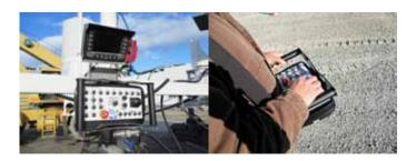
The rugged EGON Belly Pack console provides tremendous flexibility to the operator. The operator has the option of strapping on the wireless Belly Pack and working anywhere on or around the machine or docking the belly pack on a mount complete with power and LCD display. The mount can be located on the operator platform handrailing or at the ground level at the side of the machine.
