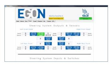
EGON IntelliMatics<sup>TM</sup> is a powerful remote diagnostics/monitoring system. The G&Z software engineering team has designed a web based remote user interface to allow maximum connectivity anywhere in the world for the contractor as well as for solving challenges with G&Z service personnel.
