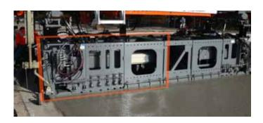
The TeleEnd: Telescopic Paving Kit End Section offers 3 ft (1m) of quick change kit per side. A 6 ft (2m) width change can be accomplished by one or two people in as little as an hour. Larger TeleEnds available up to 6.5 ft (2m) per side.
