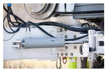
The SmartLeg system allows contractors to adjust the swing leg angle on-the-fly to maneuver around an obstacle without in the track path while the crawler track stays straight ahead.
