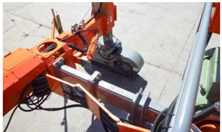
S600 hose hinge system along with a male tractor frame extension tube
