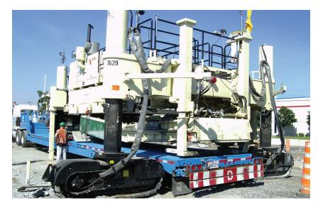
The PS1200 is designed to be transported in a single load. The PS1200 can self-load by walking over the top of the deck of a special trailer or self-load by straddling a trailer. With optional rotary actuator steering, the four track PS1200 can walk and steer on a trailer with a removable gooseneck. To reduce weight for interstate transport, the Strike-off / Spreader Plow module as well as the conveyor can be removed.
