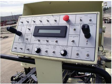
Networked Microprocessor Control System runs all the machine's control system including: proportional manual and automatic elevation and steering controls, elevation control on all four corners of tractor, self-diagnostic capability, anti-twist control, triple cross control, counter rotation capability, 90 degree steering mode on four track version, remote engine low idle switch, constant system monitoring of all sensors, and strike-off height, skip height and angle controls.
