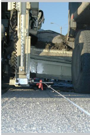
Electronic, no contact type, moisture proof, and proportional Sauer Danfoss (SD) steering and elevation sensors, as well as G&Z's own proprietary software provides precise steering and elevation accuracy and self-diagnostic capability.
