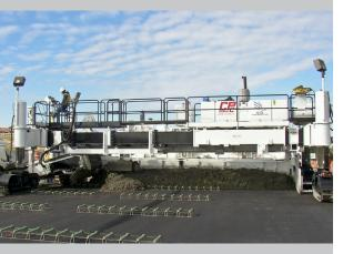
The PS1200's heavy duty tractor frame with 7'-0" (2.13 m) telescopic ability capable of 18'-0" to 25'-0" (5.50 m to 7.60 m) spreading widths. With extensions, spreading widths of up to 41'-0" (12.5 m) are possible. Its narrow profile design requires only 25" (635 mm) of trackline. A telescopic hose/cable tray is provided for paving widths from 18'-0" to 29'-0" (5.50 m to 8.80 m). Extensions are available for narrower working widths.
