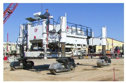
Optional 90 Degree Steering allows the four crawler tracks to be turned perpendicular to the paving direction with a flip of a switch. There is a limited steering range in this mode. 90 Degree Steering reduces the size of hand pours, dramatically increasing on site placer maneuverability and helps speed width change and self-loading for transport.
