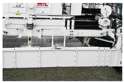
The Strike-off has the ability to crown at the centerline or off centerline with the optional hydraulically powered 6'-0" (1.8 m) crowning section for up to a maximum of 4" (100 mm) crown height. The crown section is capable of inverting as well. The Strike-off crown section includes a scale and hydraulic controls that are remotely controlled by the operator.
