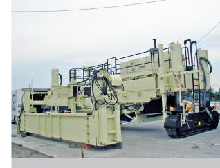
Working in conjunction with the tractor's ability to quickly counter-rotate within its width, the patented Rapid Belt Relocation system allows rapid change of the PS1200's feed side. The PS1200's Strike-Off / Spreader Plow module mounts in less than 2 hours on the front or back of the tractor for right or left hand feeding. With the patented Belt Relocation system, no crane is required.
