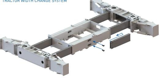
By sliding the easy to add JC Tractor Extender Sections (two pins per section) into the tractor center module tunnels, and pinning the extensions to the ends of the male telescopic tubes, the tractor frame telescopic range quickly increases from 18ft to 34ft (5.5m to 10.4m) without the time consuming need to bolt-in, tractor frame extensions or disconnecting hoses. The tractor frame can be telescoped by turning the crawler tracks in the 90 degree mode and walking the frame together or apart.
