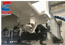
Hydraulic clamping pucks are available in lieu of mechanical pucks as an option to quickly and easily change width on the double telescopic tractor frame.
