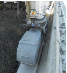
The S850SL has the narrowest bolster profile in its class. With optional 9" (228mm) wide grousers only 12" (305mm) is needed from the toe of the barrier wall to the inside edge of concrete!
