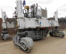
The AccuSteer system offers unparalleled maneuverability and accuracy allowing synchronized steering in 90 degree mode in every swing leg position. The SmartLeg system in tandem with AccuSteer, allows the swing leg angle to be adjusted on-the-fly to maneuver around an obstacle while automatically keeping the crawler track straight ahead. These two systems also allow rapid and semi-automatically reconfiguration of the machine into the transport configuration.
